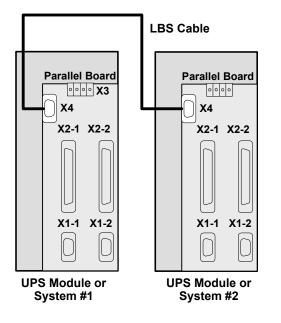
The parallel board is on the interior of the Liebert<sup>®</sup> NX<sup>™</sup> UPS, above and left of the power electronics; see Figure 29.
